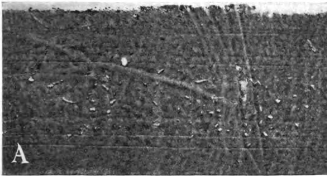
Fig. 1 (A)—34 x 4 Continental tire inflated to 35 pounds pressure per square inch showing holes and cuts that need filling
